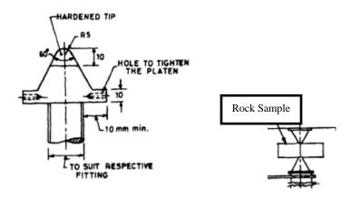
o **Loading plates:** Loading platens shall be conical with 60° angle and the radius of curvature of the cone truncation shall be 5 mm as shown in Fig.
